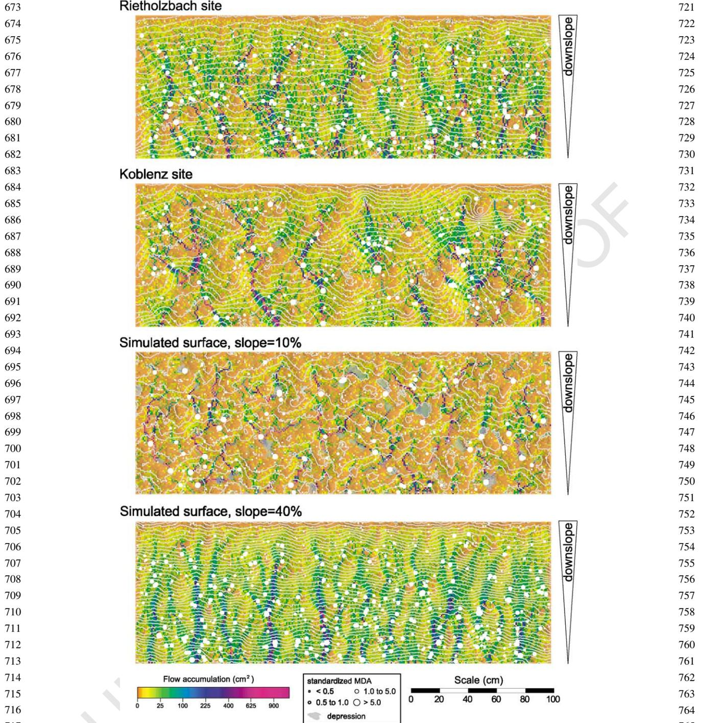
718 Fig. 1. Flow accumulation pattern at the soil surface for two surveyed sites (Rietholzbach and Koblenz) and for two simulated surfaces. Grey
